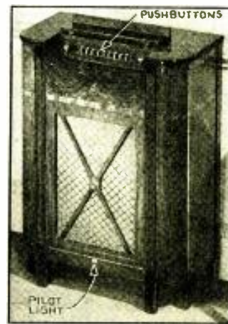
RCA-VICTOR Symphony model HF-1 high-fidelity receiver. There are no dials. Eight stations are pre-tuned and set for automatic pushbuttons. A 9th button turns the instrument off. Uniform reproduction of from 50 to 7,000 cycles, with a peak output of 12 watts is claimed.
