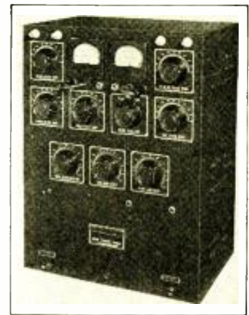
Fig. A. Front view of the band-switch 5-, 10- and 20-meter transmitter.
